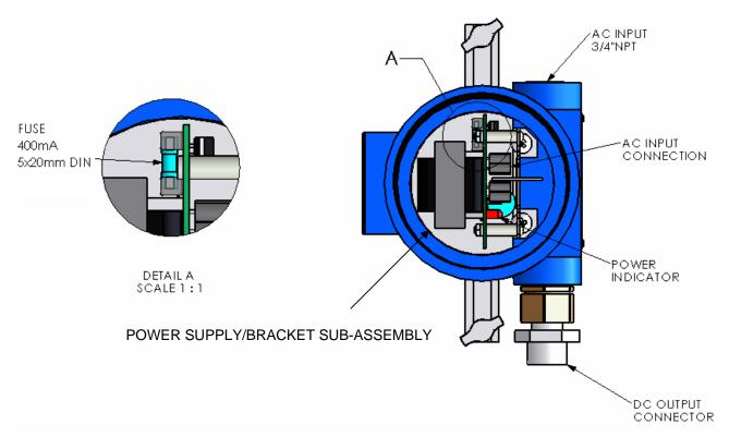
CAUTION: Incorrectly wiring the AC input to the DC output will cause permanent damage to the power supply and result in the ignition of hazardous atmospheres.
