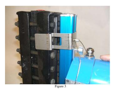
**Step 2:** Press LumaStar assembly against rear of gauge as shown in Figure 3, aligning the bracket cutouts over the gauge bolt heads as shown. Align the brackets with the  $2^{nd}$  set of bolts in from each end of the gage, when possible.
