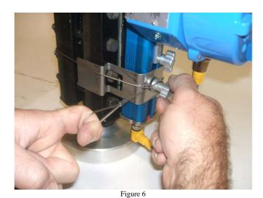
**Step 4:** Align bottom bracket, using the 2<sup>nd</sup> bolt if possible. Wrap thumb nut end of the cable around the entire gauge and begin to thread. Pull the cable loop as tight as possible and fully tighten the thumb nut down as shown in Figure 6. The lower bracket should now be tight and secure.
