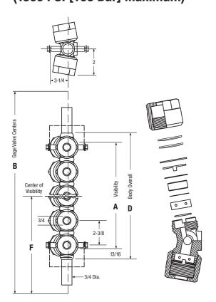
Simpliport gage connections for pressures to 1500 PSI (103 Bar) include standard nipple connections (end stems), ANSI flanges (as specified) or male/female socket welds.
