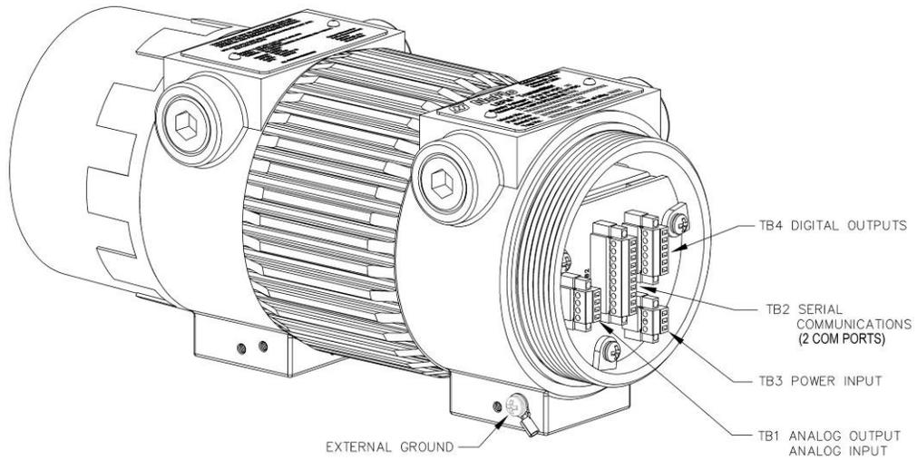
Figure 5.3: User Terminations - Cover Off (Communications Option 1)
