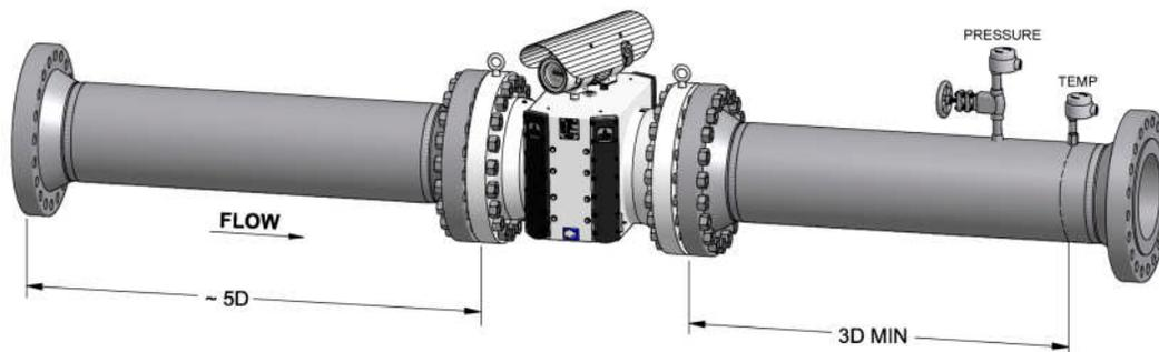
Figure 2.1: Best Practice for Installation Hydraulics
