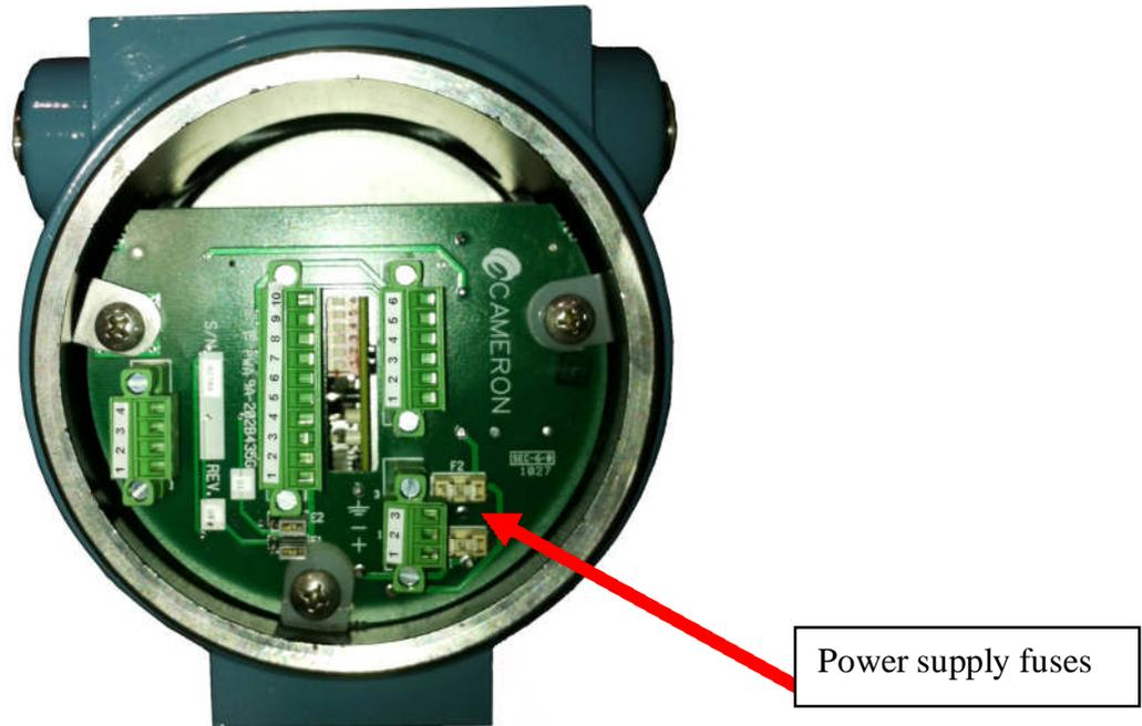
Figure 8.9: Backplane Interface Board (BIB) Fuse Location (Communications Option 1)
