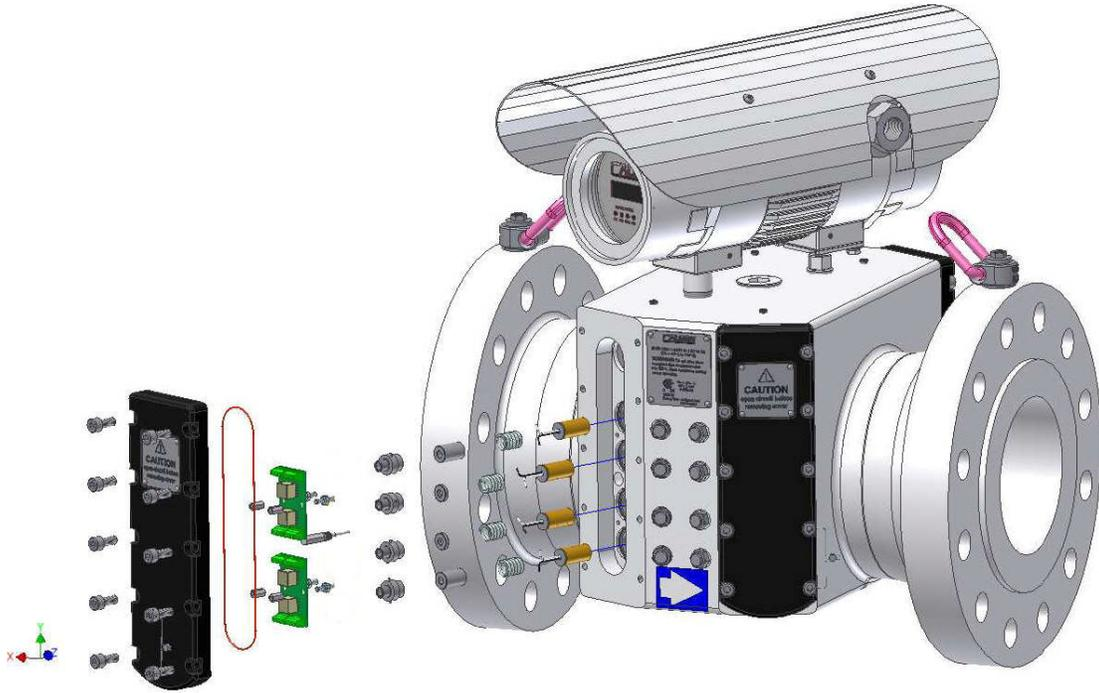
Figure 8.12: Transducer Replacement
