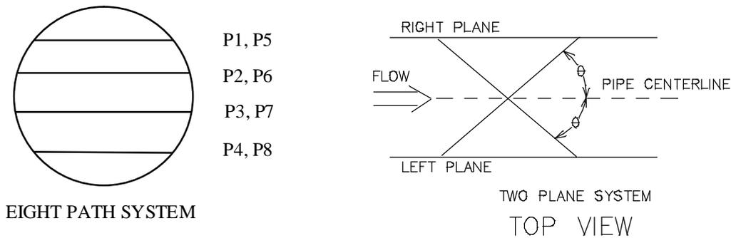
Figure 6.2: Acoustical Path Configurations
