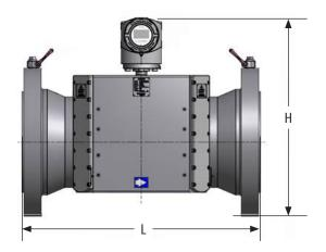
Meter body with integral transmitter
