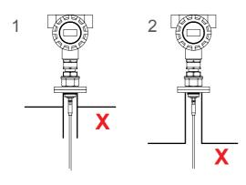
1. Stand pipes protruding into vessel may cause signal interference. Digitisation and / or Blanking Distance must be adjusted to avoid measurement issues
