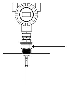
When Installing the CGR unit, use spanner or wrench ONLY at Process Fitting as indicated.
