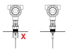
Nozzle / Socket should not protrude into vessel
