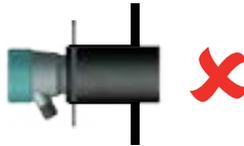
**Do not mount where sensor can be damaged by material**
