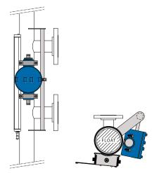
OES switch attached to switch mount rod
