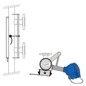
ORS switch attached to switch mount rod
