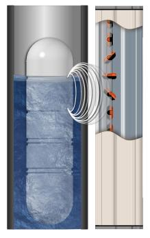
The float's 360° magnet assembly produces a strong and consistent flux array allowing visual indication through chambers as thick as schedule 160.
