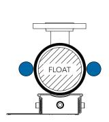
Probe mounting positions on Atlas™, Vector™, and Gemini™ magnetic level indicators.
