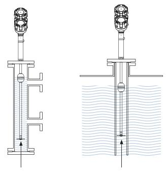
Units mounted in stilling wells or chambers are provided with centering disc at the base of the probe, guaranteeing free movement of the float.
