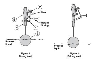
arated by a non-magnetic, pressure tight enclosing tube (5). The switch (2) and magnet (1) are assembled to a mechanism with a swinging arm which operates on precision stainless steel pivots.
