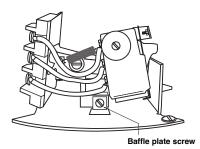
Figure 10 Baffle plate screw
