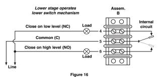
Single float with two switches or dual stage displacer
