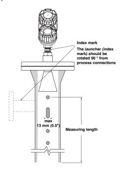
3", 4" and 6" horn antenna can be used for mounting in standpipes and stillwells. Use below table to select the right antenna for matching with the pipe size of your standpipe/stillwell.
