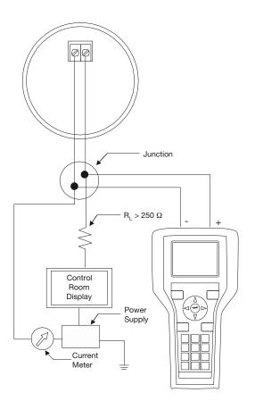
A HART (Highway Addressable Remote Transducer) remote unit, such as a HART communicator, can be used to provide a communication link to the PULSAR Model R86 transmitter. When connected to the control loop, the same system measurement readings shown on the transmitter are also shown on the communicator. The communicator can also be used to configure the transmitter.
