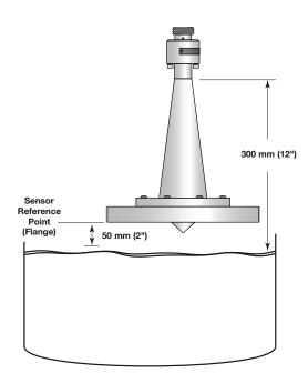
**ASME or EN Welded Flange**
