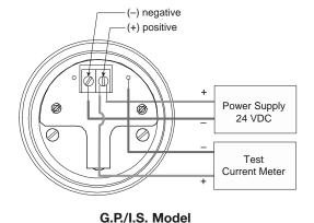
NOTE: When using a HART communicator for configuration, a minimum 250-ohm line load resistance is required. Refer to your HART communicator manual for additional information.
