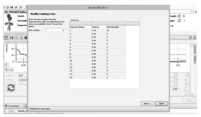
Upon presentation of the Rejection echo list (including the echo amplitudes), along with a display of the present level, select the desired false echo to be modified. (The distance to the echo must be smaller than the distance to the level echo).
