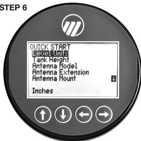
7. After making all of the necessary changes in the QuickStart menu, press the BACK button three times to return to the Home Screen.
