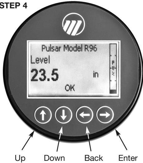
3. The push buttons offer multiple forms of functionality for menu navigation and data entry. (See Section 2.6 for complete explanation.)
