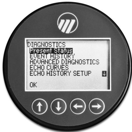
When the transmitter is operating normally and the high-light cursor is positioned on Present Status, the bottom LCD line displays “OK” because no diagnostic indicators are active.
