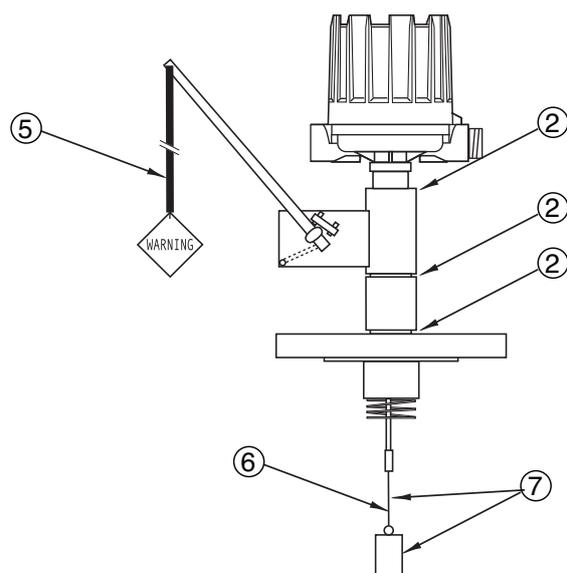
**Typical model with Proof-er and floating roof displacer**
