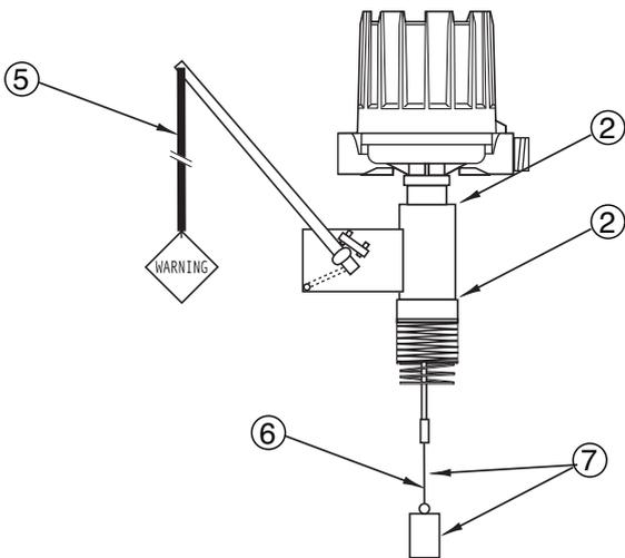
**Typical model with Proof-er and floating roof displacer**
