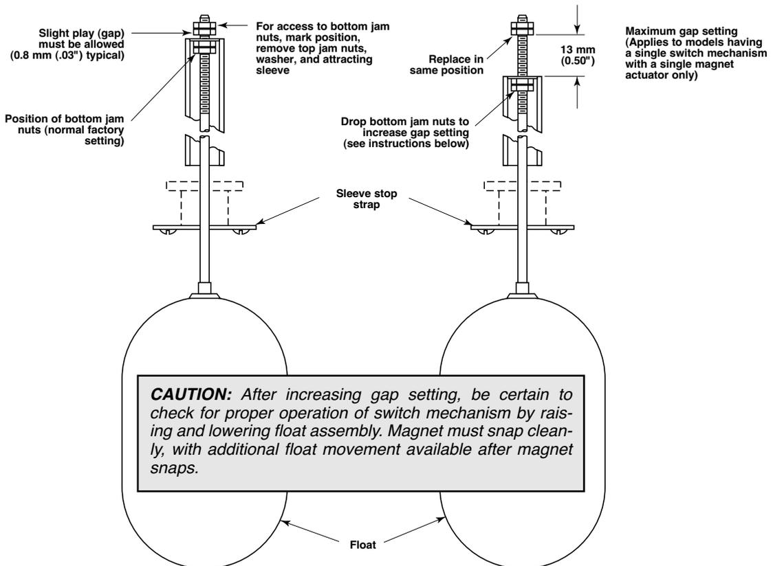
**CAUTION:** After increasing gap setting, be certain to check for proper operation of switch mechanism by raising and lowering float assembly. Magnet must snap cleanly, with additional float movement available after magnet snaps.
