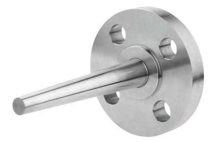
Thermowells are used to to protect the measuring instrument from corrosion, high pressure or hgih fluid velocity and to allow the measuring instrument removal for recalibration or replacement without affecting the process system. The W93 serie includes bar-stock thermowells with flanged process connection and they are suitable for heavy work conditions. These thermowells have a conic immersion length.
