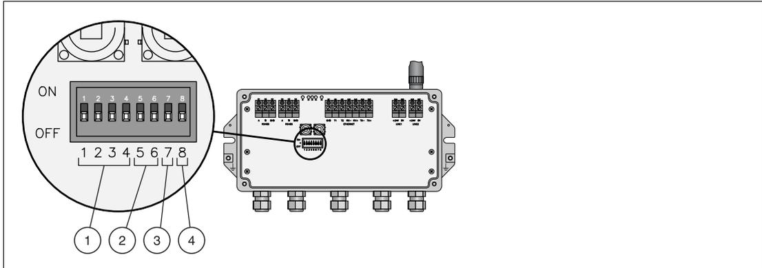
Figure 2.6 DIP switches
