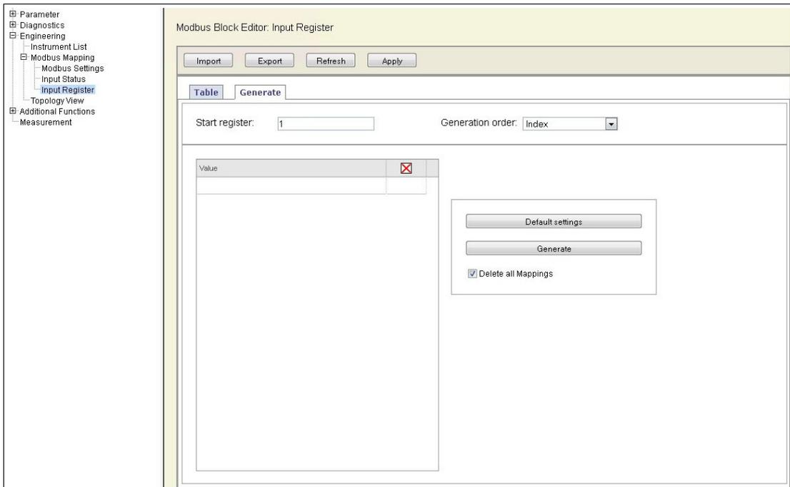
Figure 5.24 Engineering > Modbus Mapping > Input Status/Register: Semi-Automatic Generation
