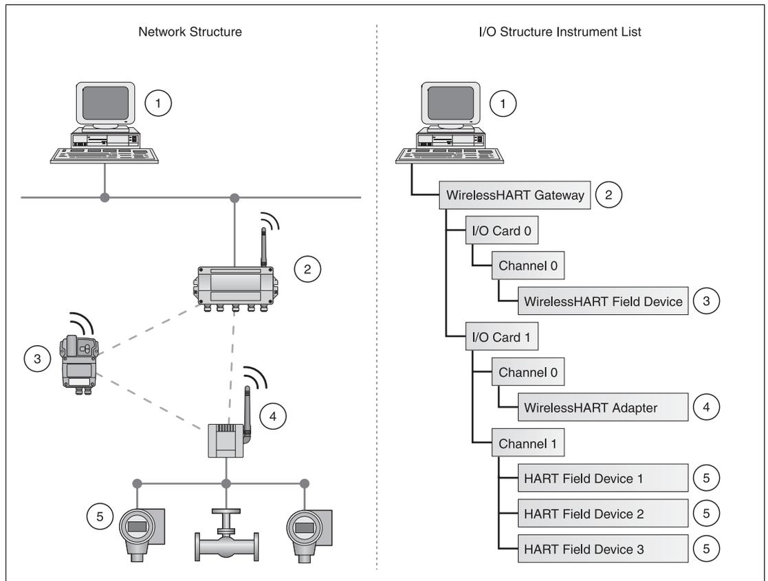
Figure 2.2 Network structure and corresponding I/O structure
