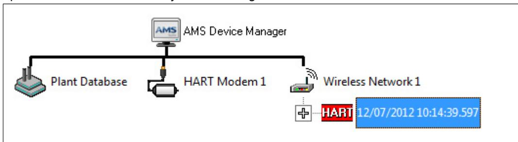
Figure 7.6 WirelessHART gateway in Device Connection View
