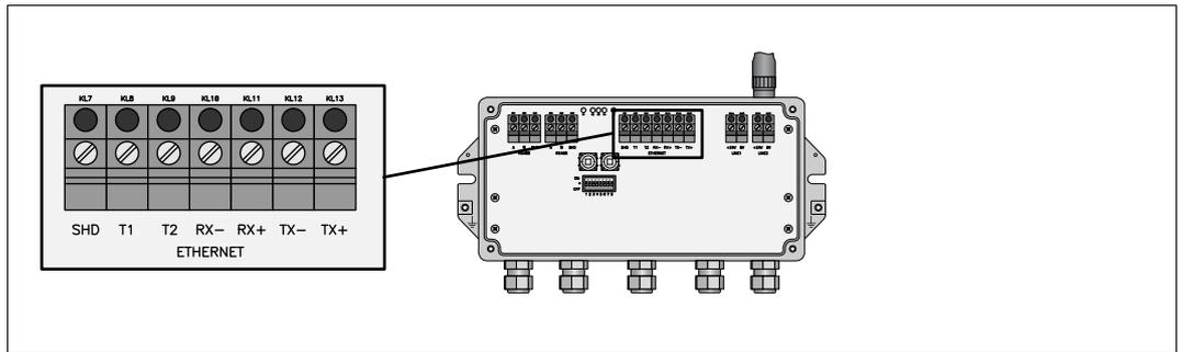
↳ The WirelessHART gateway is now connected to the Ethernet network. The yellow Ethernet communication status LED starts flashing when a correct HART or MODBUS protocol message is received.
