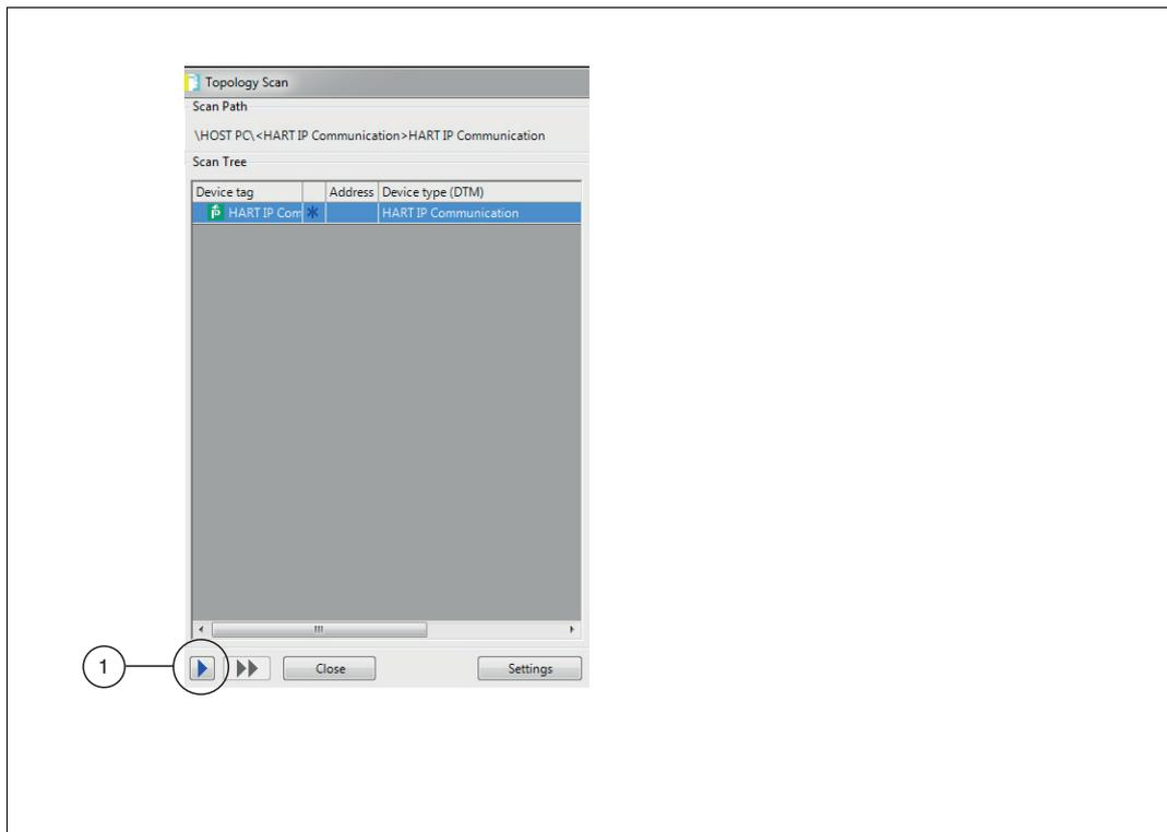
↳ Scanning is indicated by a status bar. All gateways on the network are listed. All devices that are connected to the gateways are listed. As scanning takes place, the Scan Tree section fills with all the detected participants of network, at the same time the project tree is updated.
