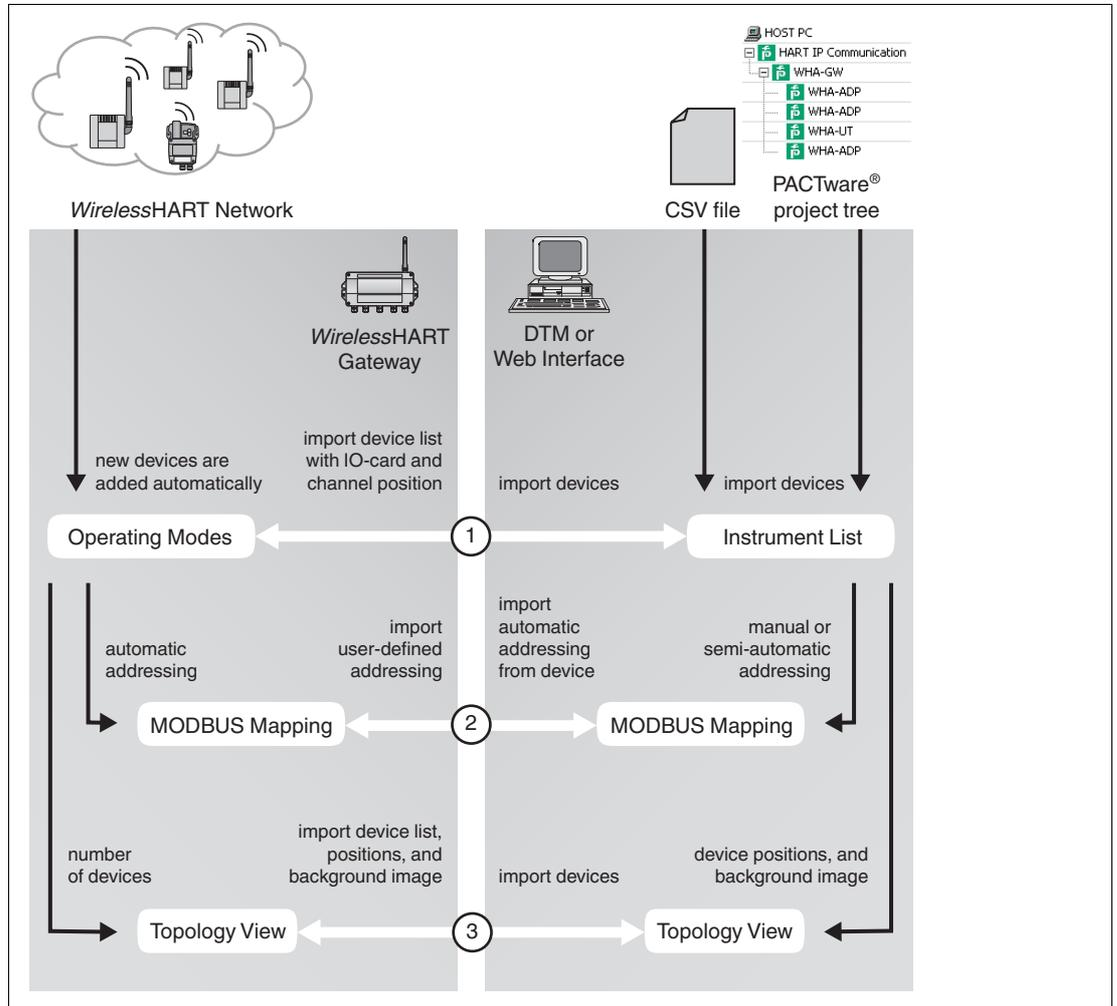
Figure 5.19 Relationship between the configuration options in the DTM or web interface and the data in the WirelessHART gateway
