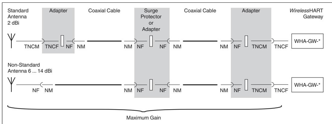
Figure 3.7 Connection diagram for standard and non-standard antennas
