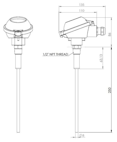
Figure 4 Structure and dimensions
