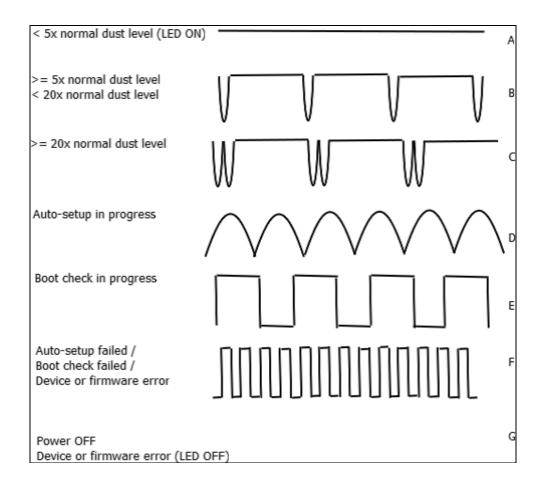
Figure 5 Description of Snifter A2 EX cover illumination sequences.
