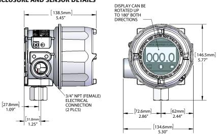
Shown with Dual Seal option M041 and gage pressure sensor
