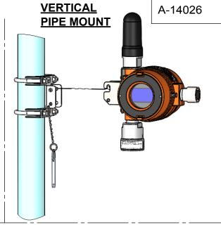
ONCE PRODUCT IS HOOKED ONTO THE MOUNTING BRACKET, INSERT THE QUICK RELEASE PIN TO SECURE.
